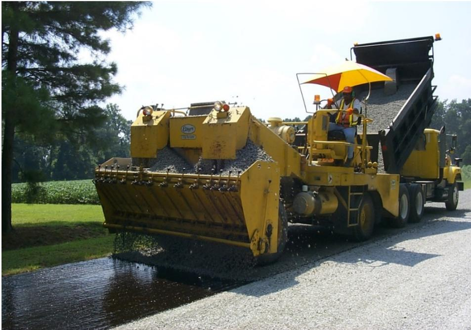
Figure 7. Stone spreader attached to dump truck.
