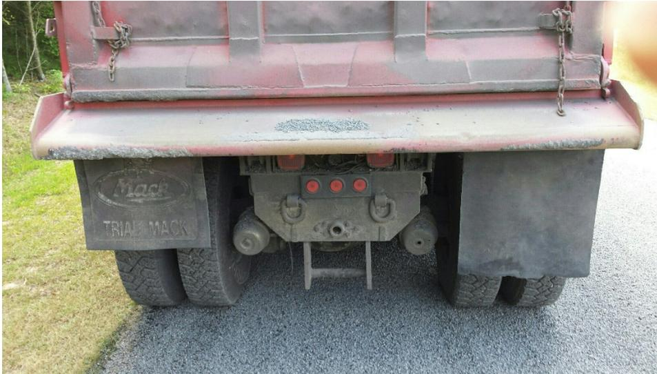
Figure 6. Dump Truck Hitch.
