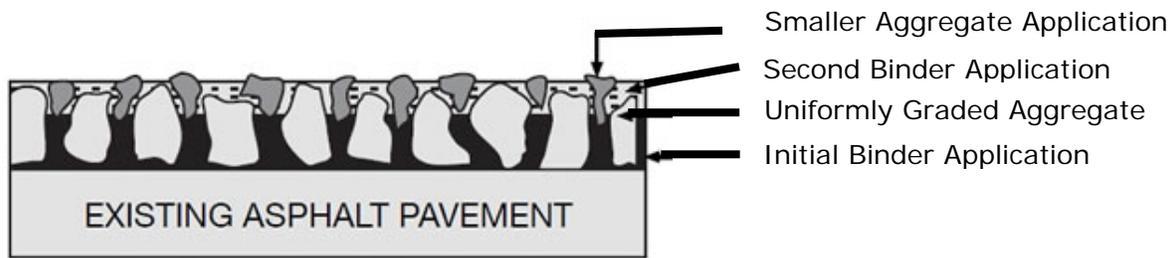
**Double Seal (2 layers of binder and aggregate)**
