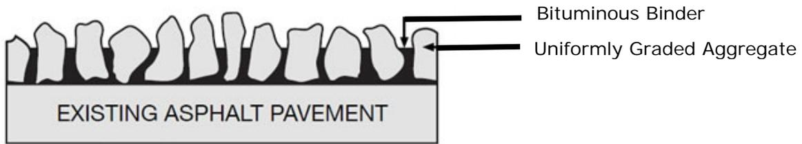
**Cross-section of a one-size seal coat aggregate**
