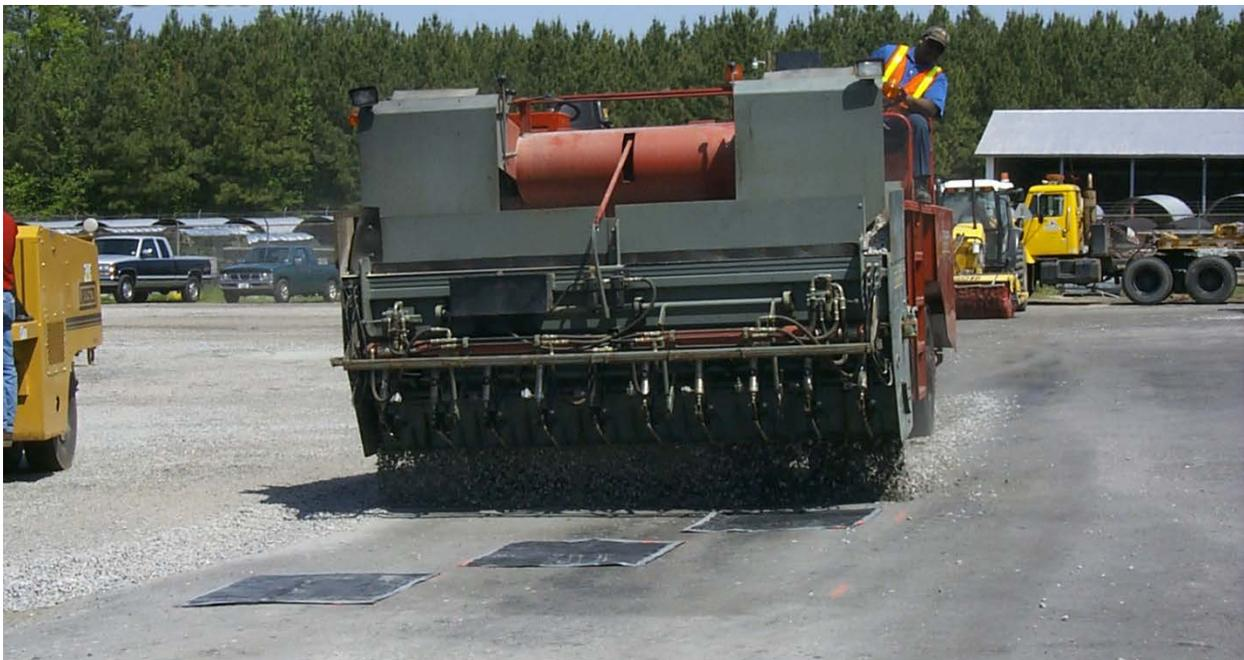
Figure 13. Calibrating the stone spreader.
