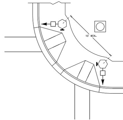
PUSHBUTTON PLACEMENT IN WIDE SIDEWALK
