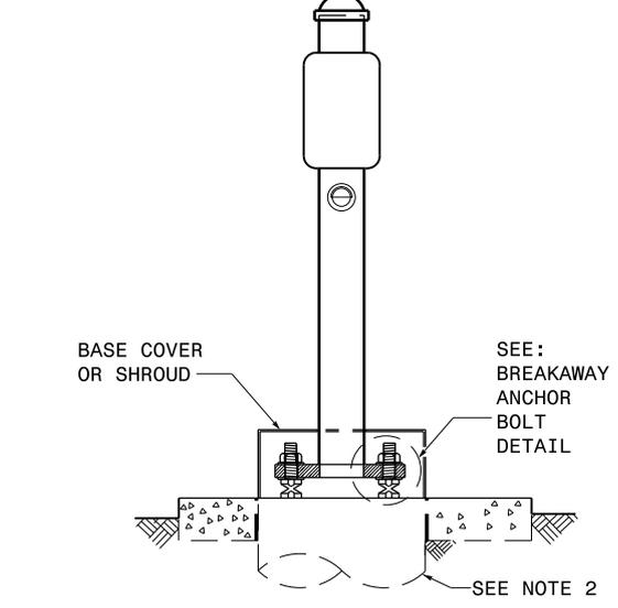
**PUSHBUTTON POST ON FLANGE BASE WITH BREAKAWAY ANCHOR BOLTS**
