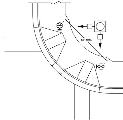
PUSHBUTTON PLACEMENT IN WIDE SIDEWALK
