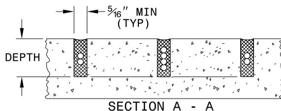
DEPTH IS 2.5" FOR CONCRETE AND 3.0" FOR ASPHALT
