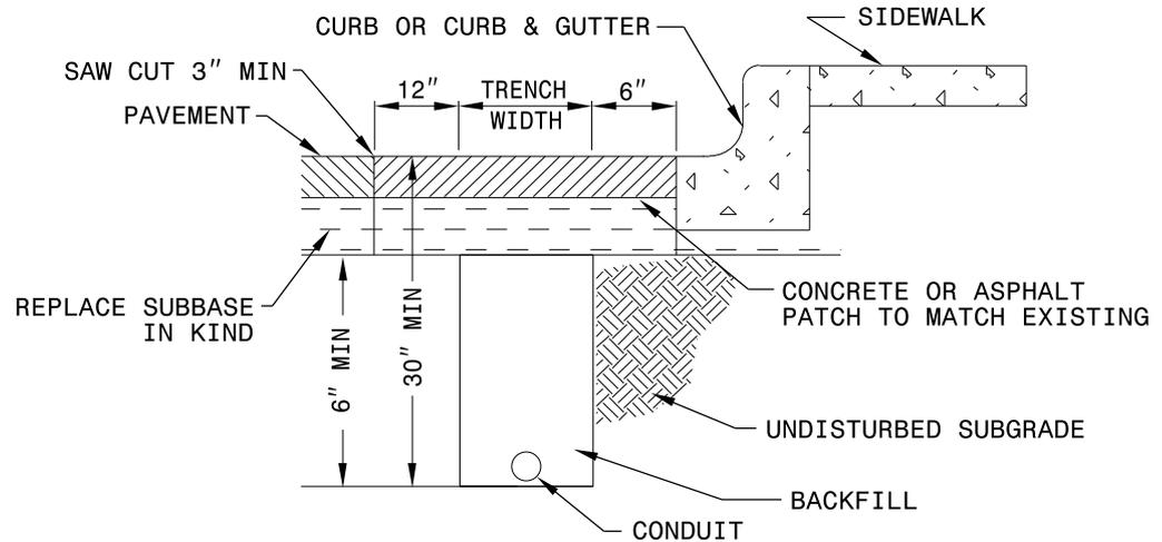
THE REMOVAL OF PAVEMENT BEYOND THE EDGES OF THE TRENCH, AS SHOWN, WILL NOT BE REQUIRED IF SAID EDGES ARE SAW CUT AND MAINTAINED NEATLY WITH NO SHATTER.
