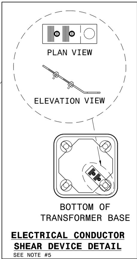
**ELECTRICAL CONDUCTOR SHEAR DEVICE DETAIL**
