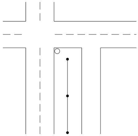
PLACE GROUNDING ELECTRODES IN A STRAIGHT LINE
