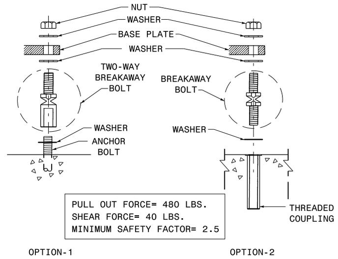
**BREAKAWAY ANCHOR BOLT DETAIL**
