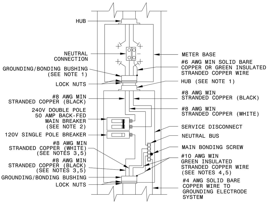
ALTERNATE ELECTRICAL CONNECTION DETAIL FOR
