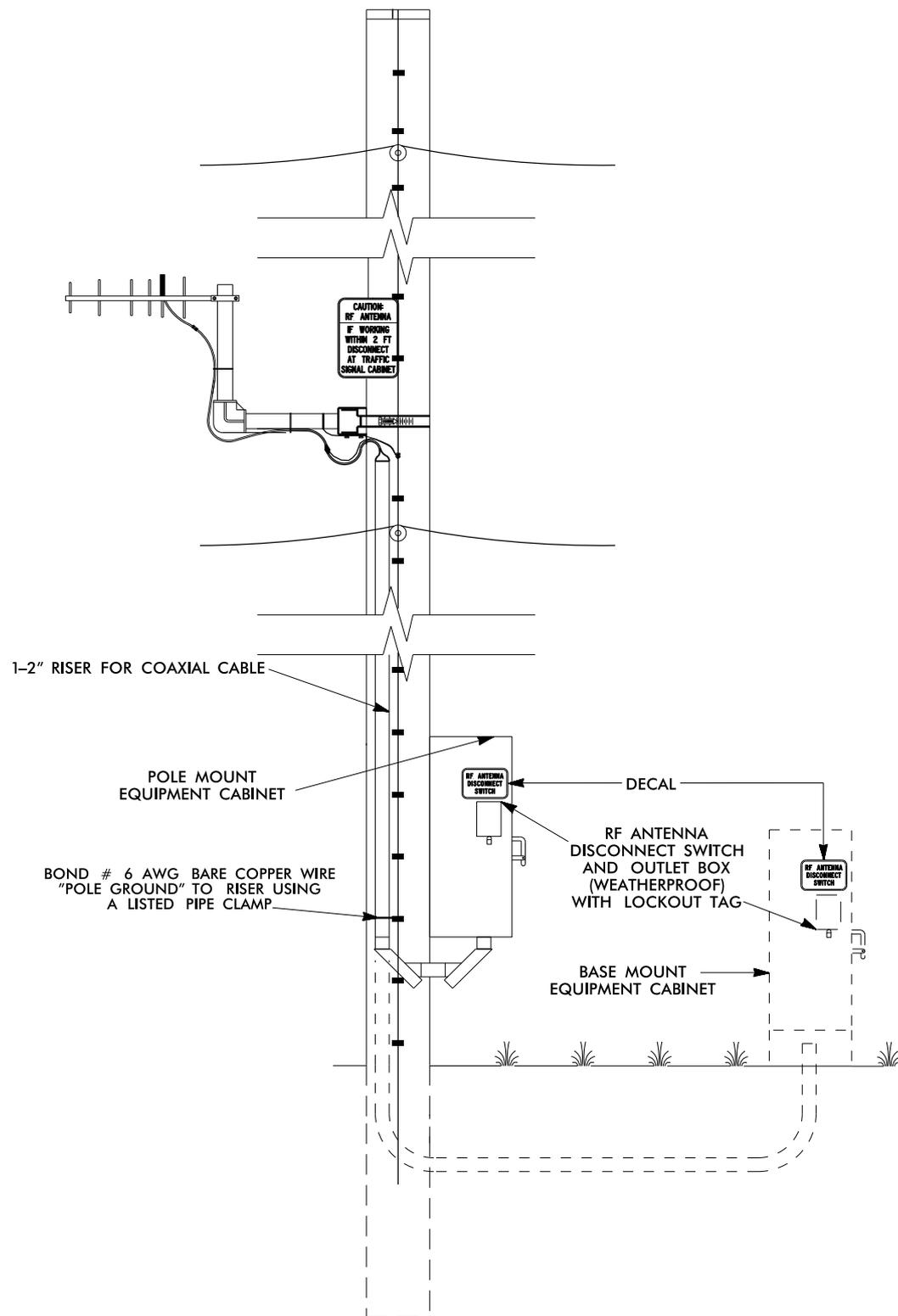
**ANTENNA AND COAXIAL CABLE CONNECTION SCHEMATIC**
